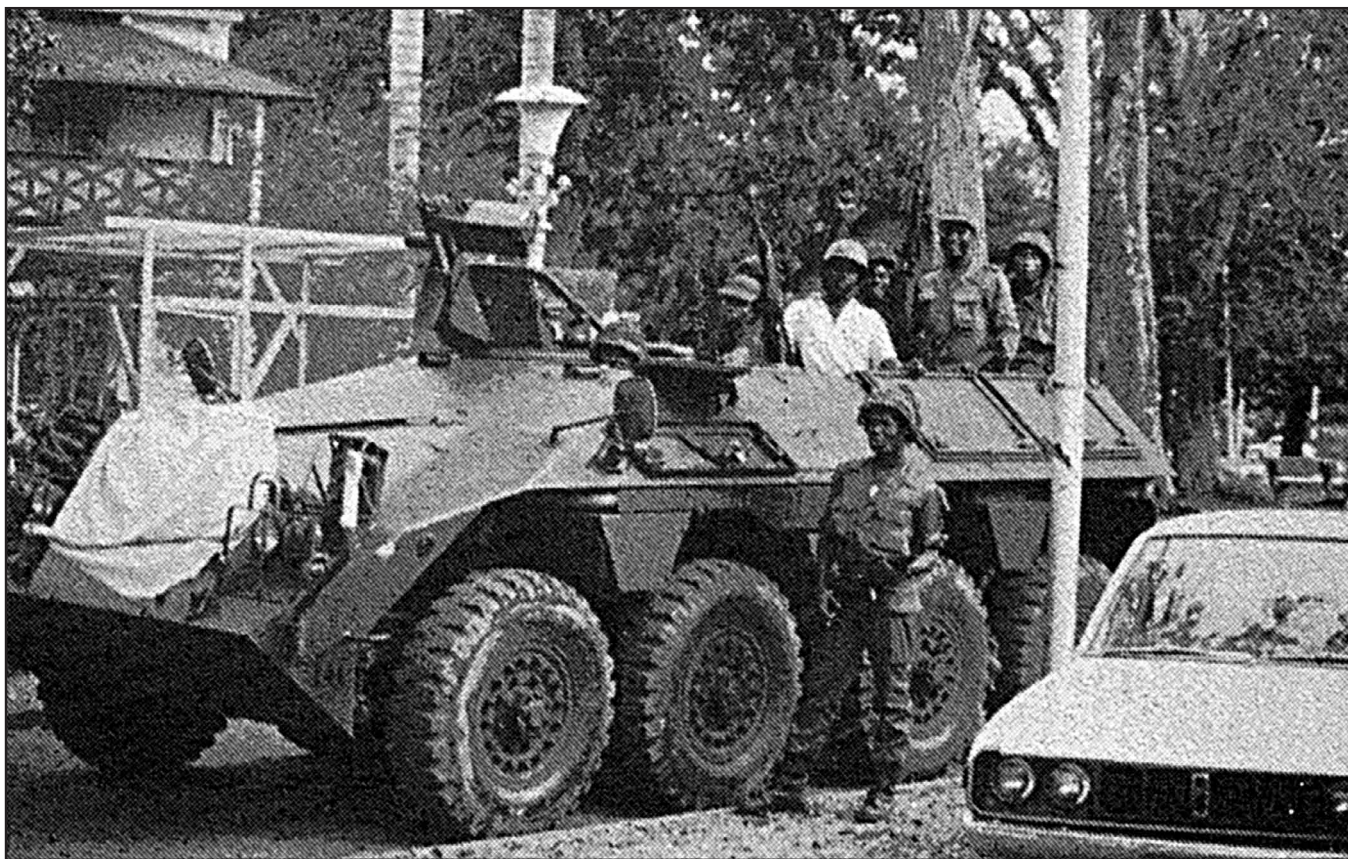
In order to distinguish the YP408s of the NBR from the ones under control of het Gezag's control, a white sheet was put onto the front of the YP to cover the title of NL. This YP408 is of the PW-V cargo carrier version, which arrived after independence. Its shortened exhaust, lack of catches for the top hatches and large indicator light distinguishes it from the YP408 that were given to the SKM when the TRIS left. (Copyright inheritors of Jul M Dubois)
