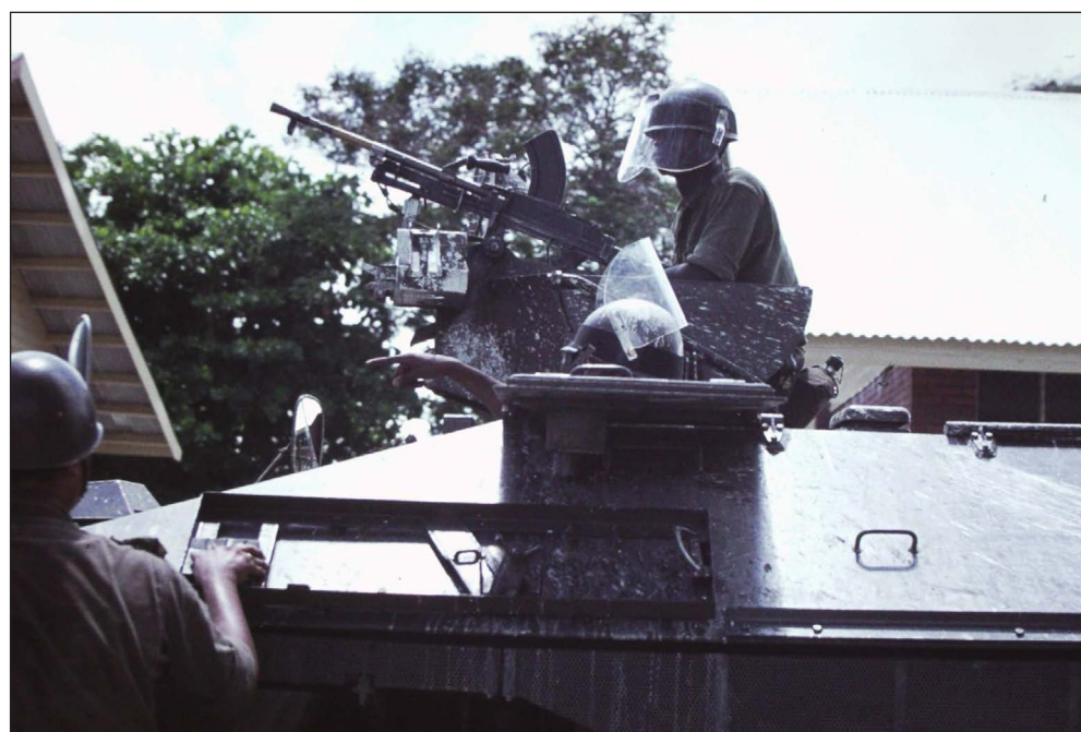
TRIS YP408s were sometimes equipped with a 7.7mm Bren LMG, probably taken from the GMC Otters. This YP408 is also taking part in a crowd control exercise. (Han van Amersfoort via DAF YP408 website)
