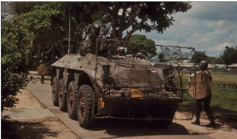
YP408 KN 75-32 equipped with a barbed wire barrier for crowd control. (Han van Amersfoort via DAF YP408 website)
